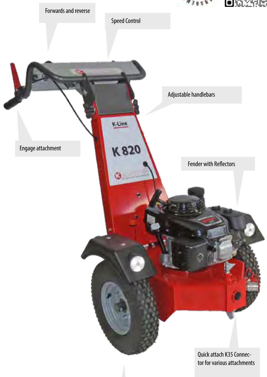
Large pneumatic tyres ideal for large obstacles such as rocks and kerbs
