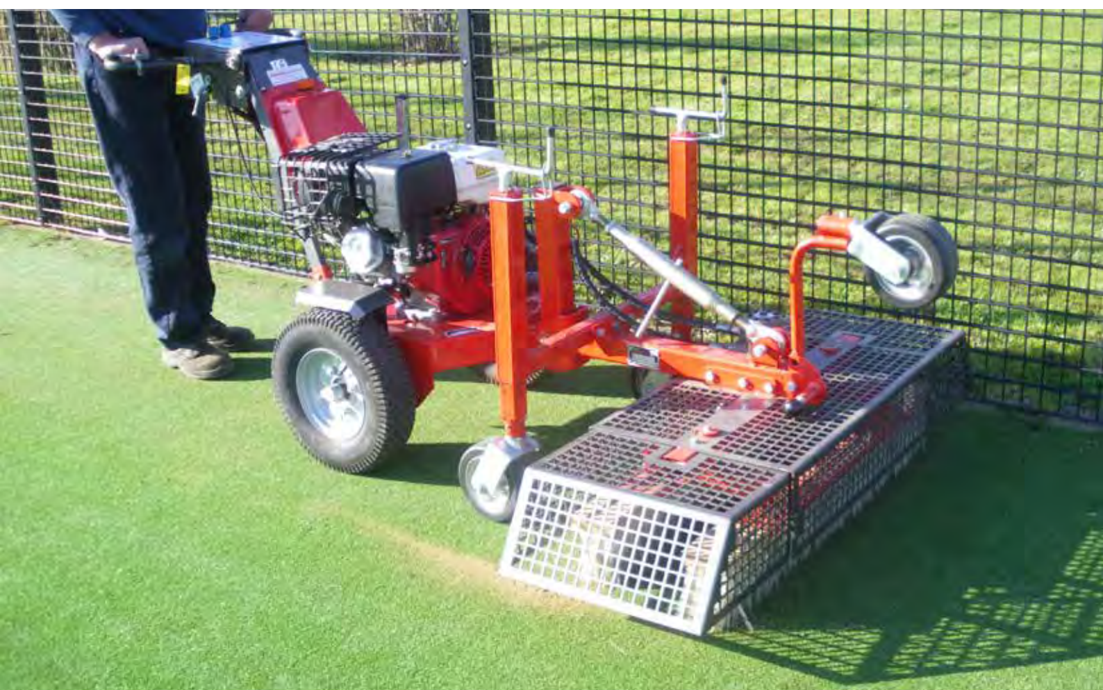
KERSTEN POWER UNIT WITH RECIPROCATING BRUSH
